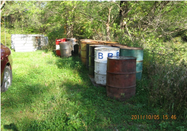
Improper outdoor storage of used oil containers – they are not on an impervious surface or protected from precipitation.
