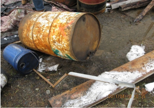
Improper storage of used oil containers
