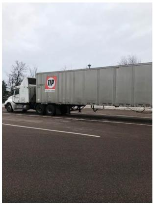
• Inspector inspected a tractor trailer at the Williston northbound detail. The inspection revealed a tire on the truck and the trailer were both severely deflated. Both vehicles were placed out of service for repair.
