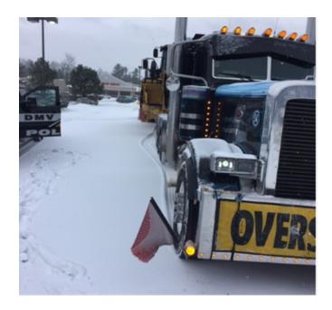
• On 11/13 Inspector conducted a level 2 inspection on a tractor trailer that had 5 flat tires. Inspection found that the operator struck a curb and the outer right tires were compromised.
