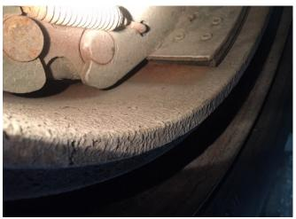
• 10/2 Lyndonville detail. An Inspector conducting a Level 1 inspection of a two axle hydraulic CMV placed it out of service for defective brakes. Both steer axle brake rotors had severe rust across the brake pad lining interface area.
