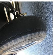
• 8/22 Searsburg, VT Rte 9, 1 Inspector screened 53 trucks, and checked 4 permits. Five inspections were completed resulting in 12 violations and 1 vehicle placed OOS. One CMV was placed OOS for several air lines with leaks at other than proper connection and, unable to pass air drop test. Driver holding brake hose which was going to steering axle brake canister had large hole in line.
