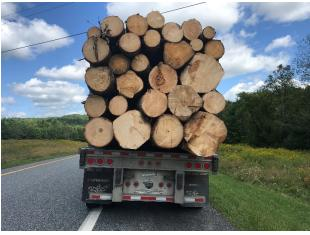
• 8/22 Inspector inspected a tractor trailer that was hauling an oversize load, which did not have the boom secured or meet the minimum tie down requirements for the weight. The vehicle was placed out of service until the defect was corrected.
