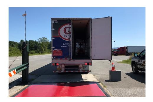
• 8/21 Inspector stopped a tractor trailer for speeding north on VT Rte 22a in Orwell. An inspection was conducted and the trailer was placed out of service for a flat tire and for having 2 loose wheel fasteners on a spoke wheel.
