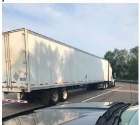
• 7/10 Inspector inspected a tractor trailer at the Williston detail. The trailer was placed out of service as tire was leaking air from a piece of metal stuck in it. The carrier was ticketed for the violation.
