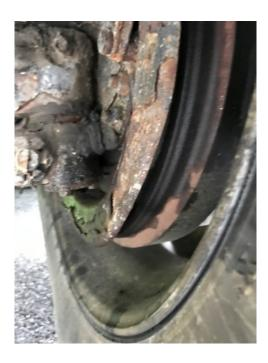
6/25 Inspector observed worn and missing bushings along the suspension system on a trailer.
