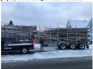
• 2/13 Inspector stopped and inspected a CMV transporting logs on US Rte 5 in Derby. There was no load securement present and the CMV was not displaying a current annual inspection. A total of seven violations were noted, two of which placed the CMV out of service. A ticket was issued to the company.
