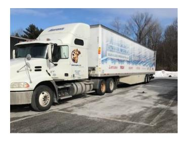
• 2/20 Inspector inspected a tractor trailer at the Georgia detail. The truck tractor was placed out of service as a hub assembly was not plugged or covered and was exposed. The trailer was placed out of service as there were 3 broken adjacent cross members. The carrier was ticketed for the hub violation.
