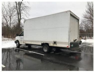
• 12/31 Inspector inspected a delivery truck hauling hazardous materials at the Williston detail. The vehicle was placed out of service for a defective parking brake. The carrier was ticketed.
