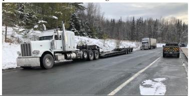
• 1/3 Inspector stopped and inspected a CMV transporting a trailer on I-91 in Derby. A Level 2 inspection was completed. The CMV was placed out of service for a defective frame and cross member. The defective cross member was supporting the upper fifth wheel plate.
