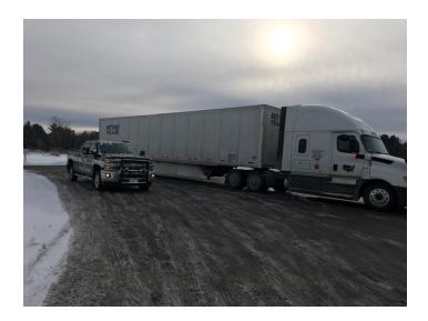
• 1/22 Inspector stopped a utility truck hauling an equipment trailer on US Rte 2 through Colchester for an equipment infraction. A subsequent inspection revealed the emergency break away system was defective. The trailer was placed out of service for repair.
