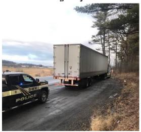
• 1/16 Inspector stopped a tractor trailer for speeding, 65mph in a 50mph zone, on VT Rte 22a in Shoreham. An inspection was conducted and the truck tractor was placed out of service as a tire was leaking air from a hole created by a screw. The carrier was ticketed for the violation.
