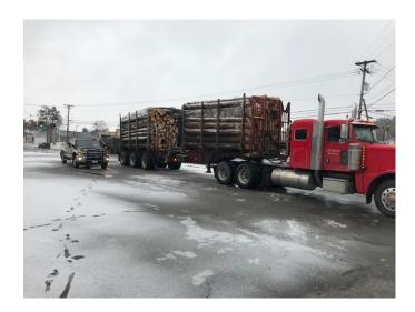
• 1/15 Inspector stopped a tractor trailer for speeding on VT Rte 22a in Shoreham. An inspection was conducted and the trailer was placed out of service for having 3 adjacent floor cross members broken.
