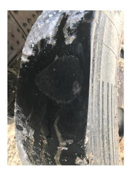
• 1/17 Inspectors responded to I89 in Milton for a report of a tractor trailer which was on fire. Upon arrival it was found the trailers brakes had caught fire, as a malfunction during transit caused the brakes to apply. A level 2 inspection was completed and the vehicle was placed out of service and towed from the roadway.
