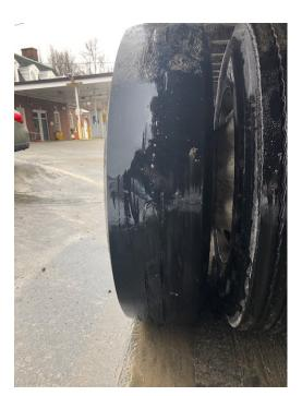
• Defective fuel tank on a two axle CMV. The fuel was seeping but was not dripping resulting in a violation but not an out of service violation.
