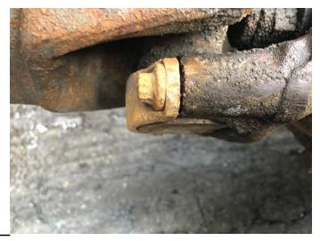
• A brake supply hose had become loose and was chaffing on the frame and brake components. Violation did not meet the out of service criteria.
