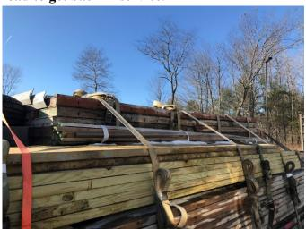
• 11/22 Inspector inspected an intrastate tractor trailer at the Cambridge detail. The vehicle was placed out of service until the loose chains on the trailer deck were secured.
