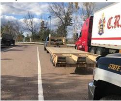
• 10/23 Inspector inspected a tractor trailer at the Williston detail. The truck was placed out of service for an air leak not at a proper connection and the trailer was out of service for inoperative stop lamps. The carrier was issued a ticket.
