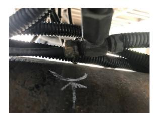
• 9/8 Inspector discovered a trailer with several audible air leaks at proper fittings. Two of four rear air canisters were leaking at their respective proper fittings. The CMV was able to maintain air pressure and was not placed out of service.
