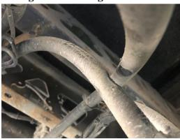
• 9/7 Wells River, US Rte 302. An Inspector conducting a Level 1 inspection placed the CMV out of service for a loose pitman arm on the steering box output shaft. As seen below, the Inspector noticed the Inspector's best friend, DPR (dry powdery rust), around the union and verified it was loose during inspection.
