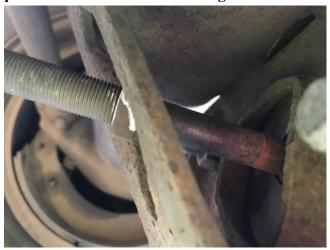
• 9/10 Inspector discovered a CMV that met the 20% OOS brake criteria. The CMV was found to have several brakes out of adjustment, active oil leaking which contaminated the inner and outer wheel surfaces on the left and right sides of axels 4 and 5. Two of the four rear wheel hubs did not contain a measurable amount of oil due to the leaking. The CMV was placed out of service for multiple violations.
