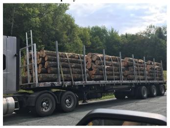
• 9/7 Wells River, US Rte 302. An Inspector conducting a Level 1 inspection placed the CMV out of service for defective suspension components. The U-bolts securing the axle to the suspension were loose.
