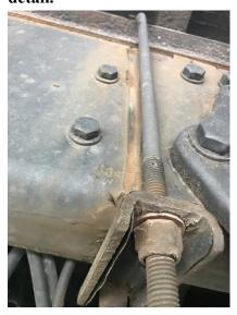
• 9/7 Inspector discovered chaffed/ degraded air lines at the Bridgewater detail. The reinforcement ply was not yet visible.
