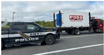
• 9/8 Inspector inspected a tractor trailer at the Fair Haven detail. The inspection revealed multiple excavators were not secured properly on the flatbed trailer. The trailer was placed out of service until the driver properly secured all four corners of the machine with 4 binders.
