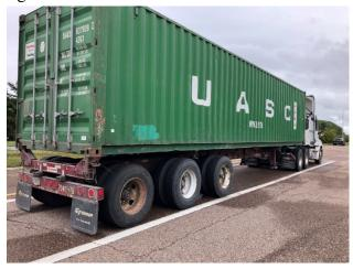
• 9/6 Inspector stopped an intrastate oversize load on I89 in Williston for a load securement violation. The hydraulic arm on the cargo was not secured. The aggregate working load limit of the tiedowns failed to meet the minimum of half the machine weight. The trailer was placed out of service until the load was properly secured.
