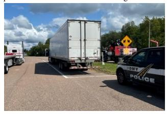
• 9/7 Inspector inspected a box truck at the Colchester detail. Multiple brakes were found to be out of adjustment on the truck, in excess of 20% of the service brakes. The truck was placed out of service for the defects.
