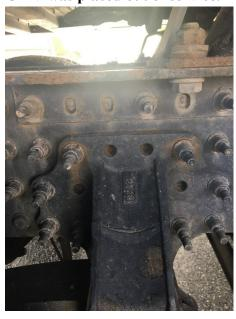
9/29 Ferdinand, US Rte 5. An Inspector conducting a Level 2 inspection of a CMV discovered a crack in the frame. The spidering crack area had been sprayed over with bedliner material in an attempt to conceal the defect. The CMV was placed out of service and the carrier was issued a ticket.
