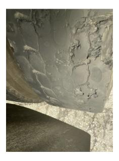
• 9/27 Inspector placed a trailer out of service for a chaffed air brake hose. The chaffing had damaged the reinforcement ply.
