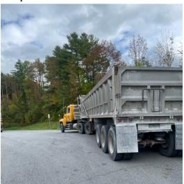
• 9/27 Inspector inspected an interstate truck and trailer at the Ferrisburgh detail. The trailer was placed out of service as one hub cover was missing, allowing an open view into the hub assembly.
