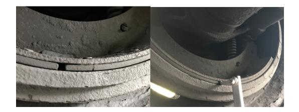
• 9/23 Inspector discovered an inoperable brake on a CMV's trailer while conducting a level 1 at the Springfield detail. The push rod was found to be completely detached from the slack adjuster. The CMV was placed out of service for the 20% brake rule after 4 of 10 brakes were found to be inoperable.
