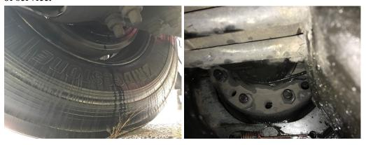
• 9/23 Inspector discovered a CMV with a worn brake lining at the Springfield detail that, measured less than 1/4" it also displayed a cracked loose segment of the lining. The CMV was placed out of service for multiple brake issues.
