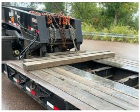
• 9/13 Inspector inspected a tractor trailer at the Williston detail. The trailer was placed out of service for having 2 wood chocks loose on the flatbed trailer. The truck tractor was placed out of service for a tire leaking air from metal in the tread.
