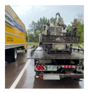
• 9/13 Inspector inspected a tractor trailer at the Williston detail. The trailer was placed out of service for having 2 large pieces of lumber loose on the flatbed trailer with no means from preventing them from falling onto the highway.
