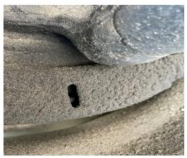
• 9/14 Inspector discovered a torn diaphragm in an air brake canister. The air leak counted towards the 20% brake criteria but did not place the trailer out of service. The trailer was placed out of service for a chaffed and damaged air hose with an audible leak.
