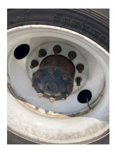
• 8/13 Lyndonville Rest Area- a six axle CMV in a truck tractor/full trailer combination came into the detail with the safety chains dragging on the roadway. An inspection was completed and the trailer was placed out of service to due a reduction in original material thickness meeting OOS standards.
