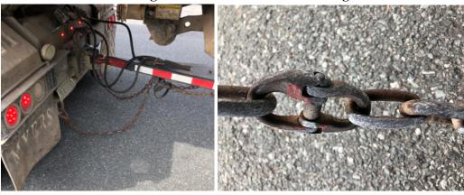
8/13 Inspector stopped a CMV on US Rte 302 in Ryegate. The CMV was placed out of service for loose cables securing the logs.
