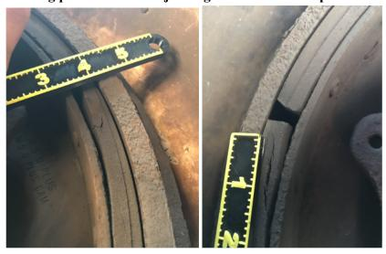
• 8/31 Inspector inspected a tractor trailer at the Williston detail. The trailer was placed out of service for no operable brake lamps, the passenger side brake lamp inoperable, and for more than 20% defective brakes.
