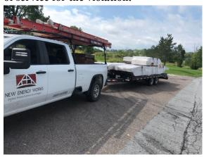
• 8/31 Inspector conducted an inspection and portable weigh on this 4 axle flatbed at the Williston detail. The vehicle was found to weigh 82,300 lbs. The road limit is 60,000 lbs. for this configuration with no permit. The vehicle was placed out of service for tires over the applicable load limit marked on the sidewall. A ticket was issued for 22,300 lbs. overweight, and the vehicle was offloaded at the detail.
