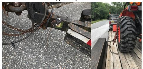
• 9/2 Inspector completed a level 1 inspection at the Sharon detail and discovered several damaged brake hoses. They did not meet the out of service criteria because the inner steel braid was intact.
