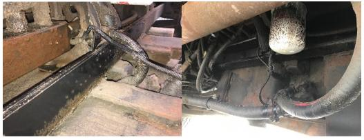
• 9/1 Inspector completed a level 1 inspection while patrolling US Rte. 4 and discovered an inoperable front right brake canister. A section of the return spring on the service brake canister was protruding out near the push rod. A total of 6 brakes were out of adjustment or inoperable. The CMV was put out of service until repairs could be made because of the 20% rule. The vehicle was being operated within in permitted weight.
