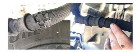
• 9/1 Inspector completed a level 1 inspection while patrolling US Rte. 4 and discovered a CMV loaded with gravel with 2 of 6 brakes out of adjustment or inoperable. The CMV was put out of service until repairs could be made because of the 20% rule. The vehicle was being operated within in permitted weight.
