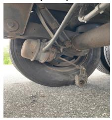
• 9/1 Inspector inspected an empty 5 axle combination and found multiple OOS violations, including brakes out of adjustment, defective tractor protection valve, exhaust leak under the cab and a rust compromised spring brake chamber. The truck and trailer were placed OOS.
