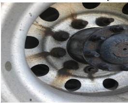
• 8/26 Inspector completed a level 1 inspection at the Randolph detail and discovered a CMV with 1 missing wheel fastener and 4 adjacent loose wheel fasteners in a 10-fastener grouping. The CMV was placed out of service.
