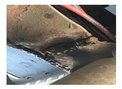
• 8/26 Inspector completed a level 1 inspection at the Randolph detail and discovered an active oil leak on the outer wheel hub. The leak did not meet the OOS criteria because it had not yet contaminated the wheel surface.
