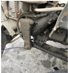
• 8/25 Inspector completed a level 1 inspection at the Springfield detail and discovered a CMV with chaffed air lines under a trailer. The damage did not extend into the reinforcement ply.
