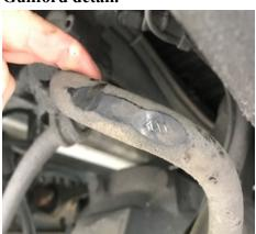
• 8/23 Inspector discovered a loose driveshaft yoke that had greater than 1/8 inch of movement with hand pressure during a level 1 inspection at the Guilford detail. The vehicle was placed out of service and repairs were made on site.
