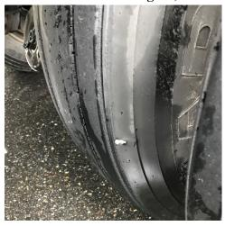
• 8/4 A tractor trailer was inspected at the Fair Haven Scale House. The trailer was placed out of service for a tire leaking air from a hole.
