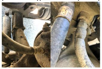
• 8/21 Inspector located a defective air brake hose on a dump truck resulting in an out of service condition.
