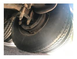
• 8/20 Inspector inspected an interstate tractor trailer at the Williston detail. The trailer was placed out of service for a flat tire.
