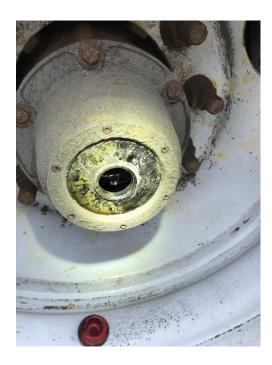
• 8/5 Inspector conducted a Level 1 inspection at the Bradford Detail on a CMV hauling a small automobile. During the inspection the Inspector discovered single load tire with metal and cord showing with a tread depth below 1/32". The trailer was placed out of service.
