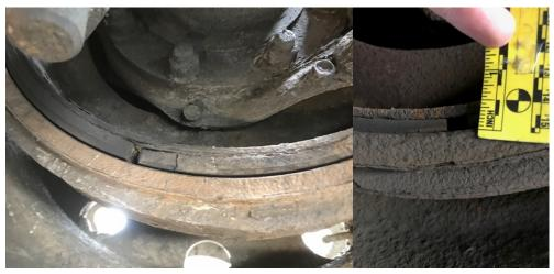
• 8/4 During a Level 1, Inspector discovered a sliding suspension system on a trailer and put it out of service for a locking pin hole that measured more than 1 inch larger than its original size. It had been previously welded but, the weld
