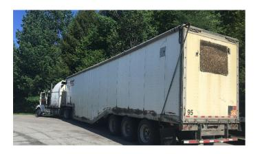
8/3 West Danville, US Rte 2. An Inspector inspected and placed a six-axle CMV transporting a large piece of equipment out of service for improper load securement- not enough chains. The driver was provided guidance and the CMV was back in service once the additional chain was added.
