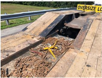
• 7/7 Inspector discovered a defective leaf assembly while conducting a level 1 inspection at the Lyndon detail. The CMV was placed out of service.
