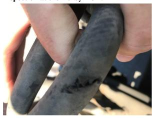
• 7/9 Inspector located an out of service emergency air hose while conducting a level 2 inspection at the Derby POE.
