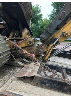
• 7/9 Inspector stopped a tractor trailer for speeding on VT Rte. 22A in Orwell. An inspection was conducted and the trailer was placed out of service for having an exposed hub assembly. Repair was previously attempted using duct tape.
