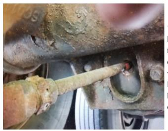
•7/7 Inspector located a loose brake lining during a level 1 inspection at the Bridgewater detail. Additionally, the inner wheel seal was also leaking but had not yet contaminated the brake friction material with oil.
