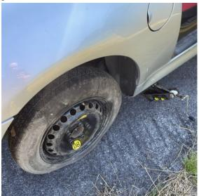
• 8/2 Inspector placed a mobile home trailer out of service at the VT Rte 279 detail for tire defects. The trailer had a flat tire and bald tire that exceeded the out of service criteria. A Level 2 inspection was completed. The driver and carrier were given warnings for the OOS violations. Violations were fixed at the scene.
