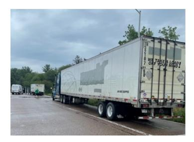
• 8/2 Inspector inspected a tractor trailer at the Colchester detail. The trailer was placed out of service for a tire that was leaking air from a screw in the tread. The truck tractor was placed out of service as the emergency glad hand hose had several bulges.
