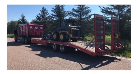
• 8/1 Inspector stopped an interstate tractor trailer on I89 in Williston that was displaying one oversize load sign. The vehicle was not oversize. The driver had forgotten to connect the trailer electrical and air lines after making his delivery. The trailer was placed out of service until the lines were connected.
