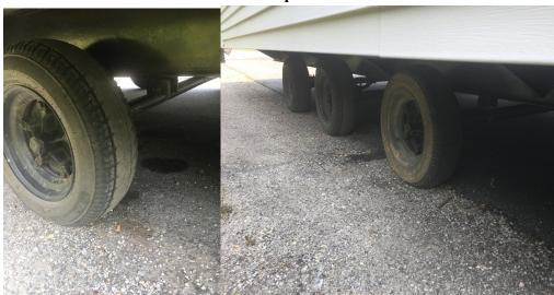
• 7/29 Inspector located this defective tire during an inspection on US Rte 7 at the Emerald Lake Pull Off detail. The tire was part of a duel set so it did not meet the out of service criteria and was documented on the inspection report as a violation only.
