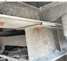
• 7/27 Inspector discovered loose upper coupler mounting bolts on a fifth wheel assembly during an inspection on VT Rte 103. Due to the loose bolts, an aluminum spacer between the trailer frame and upper fifth wheel plate had shifted out of position. Repairs were made on site and the vehicle continued the trip.
