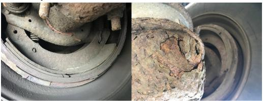
• 6/25 Inspector conducted a level 1 inspection on a tractor trailer hauling an intermodal container at the Guilford truck inspection area. The intermodal chassis had multiple brakes out of adjustment, leaking wheel seals and a tire with side wall damage. An area of the tire approximately 12 inches long and 3 inches wide had been damaged with exposed plies showing. The vehicle was placed out of service.
