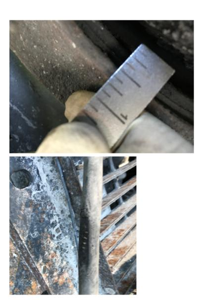
• 6/25 Inspector inspected a dump truck and discovered two loose adjacent lug nuts out of five, which caused the wheel to spin on the hub assembly at the Clarendon detail. The vehicle was placed out of service.
