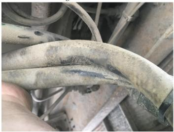
• 6/25 Inspector conducting a Level 2 inspection on a six axle CMV transporting bark mulch discovered this improper air brake supply hose on the steering axle. The recently replaced hose was not properly installed resulting in the hose being kinked and a reduction in air pressure. The CMV was also 6,500 lbs over the permitted road limit. A ticket was issued to the company.
