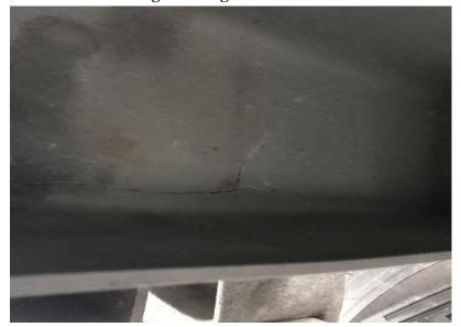
• 6/22 Inspector identified a defective rear impact guard on a trailer during an inspection at the Putney Scale House. The metal was so corroded the guard could be moved with hand pressure.
