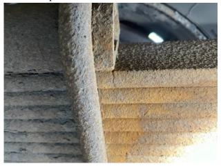
• 6/21 Inspector discovered a corroded, broken, and bent crossmember on a van top trailer. The damage did not meet the out of service criteria, but a tire was found with belt material showing in the tread area which did meet the out of service criteria and the CMV was placed out of service.
