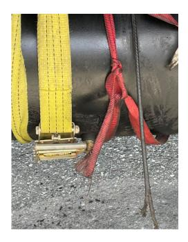
• 6/23 Inspector located a chaffed air line with damage extending into the reinforcement ply. The vehicle was placed out of service in combination only. The driver separated from the trailer and drove to a repair facility.
