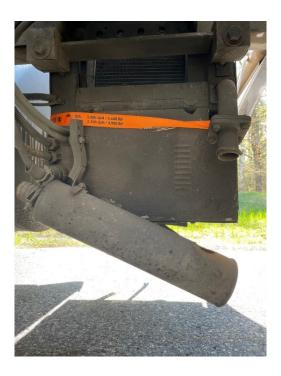
• 6/21 Inspector inspected a vehicle who came into the detail with a loose battery cover. The cover had fallen off the battery and was lodged between the gas tank and dragging on the ground. A level 2 inspection was completed, and the defect was fixed before the CMV continued its trip.
