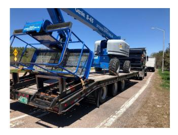
• 5/10 Inspector inspected a tractor trailer at the Colchester detail. The trailer was placed out of service as the spare tire under the trailer was not secured in it's mount.
