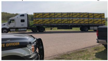
• 5/12 Inspector inspected an intrastate truck and trailer hauling machinery at the Ferrisburgh detail. A loose chain was located on the trailer deck. The trailer was placed out of service until the chain was secured.
