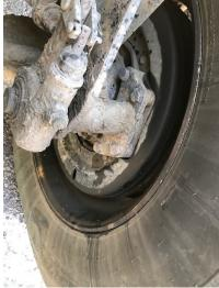
• 5/10 Inspector inspected a tractor trailer at the Colchester detail. The trailer was placed out of service as the drain valve cable on the air reservoir tank was broken between axles 4 and 5 was dragging on the ground and in between the tires.
