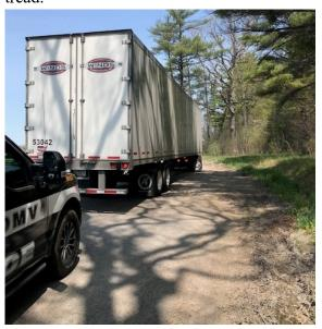
5/12 Inspector inspected an interstate tractor trailer at the Ferrisburgh detail. As the CMV pulled into the detail the rear wheels on the tractor were actively smoking. A Level 1 inspection was conducted and the combination was placed out of service for inoperable brakes.
