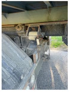
• 5/12 Inspector conduction a level 2 inspection at the Springfield detail placed a truck out of service for an actively leaking fuel tank.
