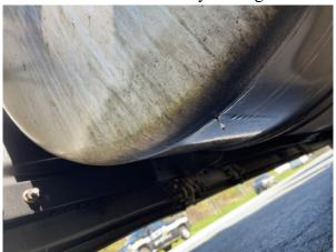
• 5/12 Inspector located a chaffed air line with the damaged area extending into the inner reinforcement plies during an inspection at the Springfield NB detail. The vehicle was placed out of service and repairs were made on site.
