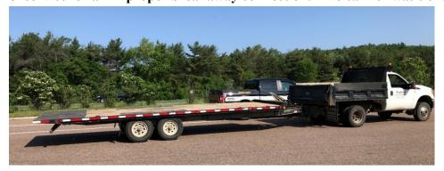
• 5/26 Cpl. Morris inspected a tractor trailer at the Cambridge detail. The operator advised the trailer was loaded with sand and presented a 99000 pound overweight permit. A measurement was taken, and the combination did not have the 51 foot axle spread required to operate under the permit as the spread was only 45 feet. A portable weigh was conducted, and the carrier was ticketed for being 9000 pounds overweight on a valid 90000 pound permit.
