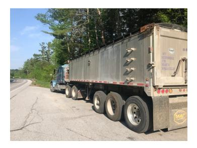
• 5/27 Inspector inspected a tractor trailer at Highgate POE detail. The inspection revealed a tire was flat on the loaded trailer. The trailer was placed out of service for repair.
