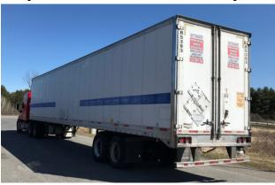
• 4/8 Inspector inspected a truck and trailer at the Fair Haven detail. The truck was placed out of service as the parking brake was inoperable. The trailer was placed out of service as the passenger side rear turn signal was inoperable.
