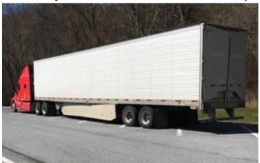
• 4/8 Inspector inspected a tractor trailer at the Fair Haven detail. The inspection revealed the rearmost stop lights on the intermodal trailer were inoperable. The trailer was placed out of service for repair.
