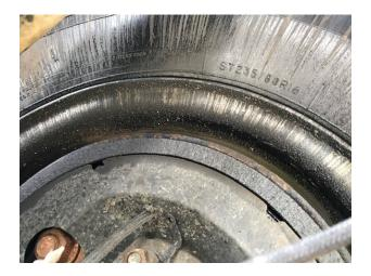
• 4/7 Cpl. Morris inspected a tractor trailer at the Ira detail. The inspection revealed the truck tractor had an air leak and failed the air drop test and the trailer had two defective tires on the same axle constituting an out of service infraction. Both the truck and trailer were placed out of service and the carrier was ticketed.
