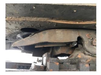
• 4/5 Inspector discovered a cracked wheel, the crack extended from the hand hole to the stud hole and the truck was placed out of service.
