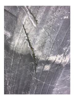
• 4/5 Inspector placed a vehicle out of service for exposed bare wire discovered during a level 2 inspection at the Ira detail.
