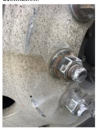
• 4/5 Inspector discovered loose U-bolts and a leaking inner wheel seal that contaminated the brake surface during an inspection at the Ira detail. The trailer was placed out of service.
