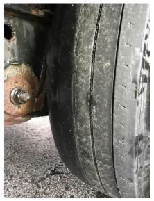
• 4/7 Inspector discovered two defective tires located in a dual set during a level 2 inspection. Both tires were worn with less than 1/32-inch tread depth remaining in two adjacent major grooves at three separate locations around the circumference of the tire. The condition did meet the out of service criteria, so the vehicle was placed out of service and repaired on site.
