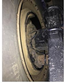
• 4/5 Inspector inspected a tractor trailer at the Georgia detail. The truck tractor was placed out of service as the axle 3 passenger side inner dual was in constant contact with a part of the vehicle. The flat bed trailer was placed out of service as there was a pile of loose dirt that was free to fly off into traffic.
