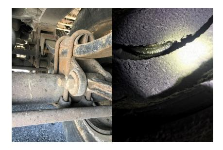
• 4/5 Inspector discovered a cracked weld during a level 2 inspection at the Ira detail. The crack was located in the hoist structure above the frame rail of a roll-off dumpster truck. The defect did not meet the OOS criteria and was marked as a violation only.
