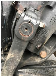
• 4/7 Inspector located a defective mount for the lower fifth wheel assembly during an inspection at the Sharon NB detail. More than 20% of the total length of all the original welds, including fore and aft, were cracked on both sides of the vehicle. The vehicle was placed out of service and repaired by a local company.
