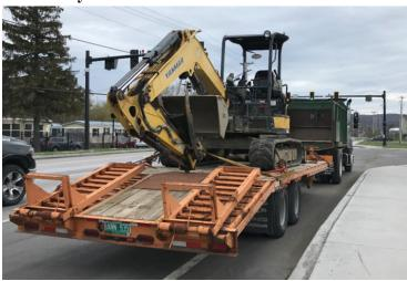
• 4/29 Inspector inspected a flat bed truck at the Williston detail. The truck was placed out of service as the parking brake was inoperable.
