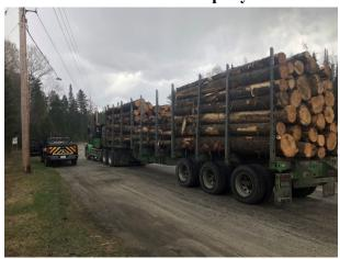
• 4/20 Morrisville detail. Inspector conducted a level 2 inspection on a log truck at the Morrisville AOT garage. Multiple violations were found including improper load securement, cracked windshield, and inoperative lighting devices. In addition, the truck was weighed with portable scales and the total gross was 10,000 lbs over the permitted weight. A ticket was issued to the carrier.
