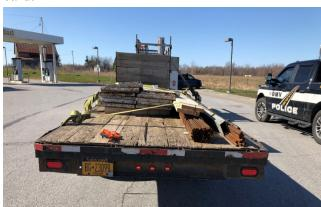
4/18 Inspector stopped a truck hauling a trailer for an equipment violation in Richmond. A subsequent inspection revealed the breakaway device was not properly hooked to the towing vehicle. The trailer was placed out of service and the driver remedied the defect.
