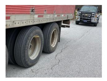
• 4/21 Inspector conducted an inspection on this combination at the Ira detail. The combination was found to require a class A CDL, and the operator had a class D license. The truck had an inoperative parking brake, and the brake lights on the towed unit were also inoperative. The driver, truck and trailer were placed out of service.
