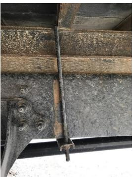
• 4/21 Inspector discovered 6 of 14 loose body mounts on a 2-axle box truck while conducting a level 2 inspection at the VT Rte. 107 Detail. The condition did not meet the out of service criteria.
