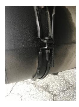
• 4/14 Inspector discovered a chaffed air hose at the Vernon detail, the air hose was chaffed through the reinforcement ply into the inner core. The trailer was placed out of service until it was repaired on scene.
