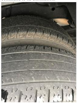
• 4/12 Inspector discovered several flat spotted tires on the trailer of a CMV while conducting a level 2 inspection at the Guilford detail. The damage was only located on half the tire which did not meet the OOS criteria. The violation was marked as a defect only.
