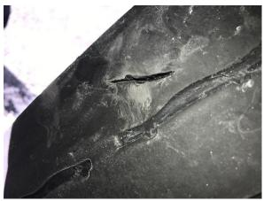
• 4/12 Inspector discovered a bald tire during a level 2 inspection at the Guilford detail. The tire was in a dual set and was marked as a violation only because the other tire did not meet the OOS criteria.
