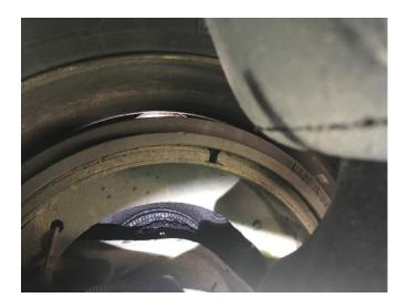
• 4/12 Inspector discovered tires worn below 2/32-inch tread depth during an inspection at the Guilford detail. The tires were in a dual set and although close did not meet the out of service criteria. The violation was documented, and vehicle continued to its destination.
