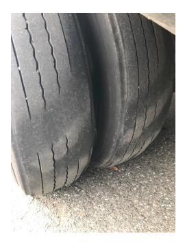
• 4/12 Inspector conducted a traffic stop on a CMV that did not stop at the Guilford detail. She discovered a cut tire with belt material exposed but it did not meet the 2" OOS criteria. The defect was marked as a violation only.
