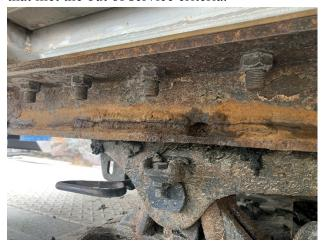
• 4/14 Hartford detail. An Inspector conducting a Level 2 inspection of a five axle CMV placed the CMV out of service for a body component contacting a tire. The support for the wheel well broke resulting in the fender contacting the tire and causing damage.
