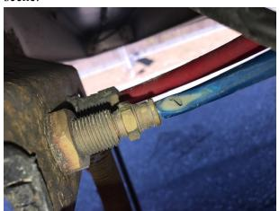
• 4/11 Inspector conducted a traffic stop on a CMV in WRJ and completed a level 2 inspection. She discovered an air hose that had been cut. The damage extended through the reinforcement ply and the truck and trailer combination was placed out of service until repairs could be made.
