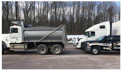
• 3/23 Inspector inspected a tractor trailer at the Williston detail. The trailer was placed out of service for a tire that was leaking air.
