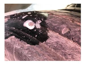
• 3/25 Inspector inspected an interstate tractor trailer at the Georgia detail. The driver was placed out of service as his CDL had been downgraded, due to lack of a valid medical card. The trailer was placed out of service for a non-manufactured hole in a spring brake can.
