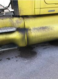
• 3/24 Inspector inspected a tractor trailer at the Ira HP detail. The inspection revealed the driver's side fuel tank had a leak which was pooling fuel on the asphalt. The truck was placed out of service for repair.
