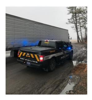
• 3/18 Inspector inspected a box truck in Shoreham. The truck was placed out of service as the axle one passenger side tire had belt material exposed.
