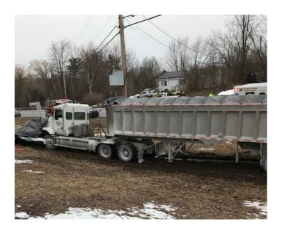
• 3/16 Inspector responded to I89 in Milton for a crash. A southbound tractor trailer dropped its driveshaft. Several vehicles got flat tires from running over the driveshaft. An inspection was conducted, and the truck tractor was placed out of service.
