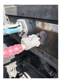
• 3/17 Inspector completed a Level 2 inspection on a 6-axle combination vehicle with an audible air leak. A pinhole was found on a secondary air tank under scaling rust; the vehicle passed the air loss rate test and did not meet the OOS criteria.
