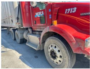
• 3/17 Inspector inspected a tractor trailer at the Georgia detail. The inspection revealed a tire was severely deflated on the truck tractor. The tire's measured psi was 50% less than the marked maximum psi stamped on the tire and the truck tractor was placed out of service for the defect.
