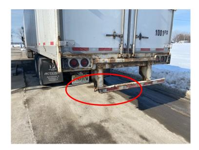
• 2/9 Inspector stopped this 6 axle log truck traveling west on US Rte. 4 in Fair Haven for a suspected overweight violation. A platform weigh at the Fair Haven Scale House found the vehicle to weigh 105,700 lbs. The carrier had a valid permit, but the trailer brakes had a malfunction resulting in the tag axle being inoperative, rendering the permit invalid. The carrier was ticketed, and the vehicle was grounded.
