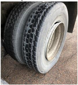
• 2/10 Inspector inspected a box truck at the Colchester detail. The truck was placed out of service as the axle 1 driver's side tire had belt material exposed.
