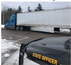
• 2/10 Inspector inspected a tractor trailer at the Colchester detail. The trailer was placed out of service for a flat tire. That tire was also completely bald. The carrier was ticketed for the violation.
