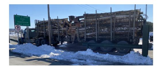
• 2/9 Inspector stopped this 6 axle log truck traveling west on US Rte. 4 in Fair Haven for a suspected overweight violation. A platform weigh at the Fair Haven Scale House found the vehicle to weigh 113,740 lbs., 14,740 lbs. over the 99K permit. The carrier was ticketed.
