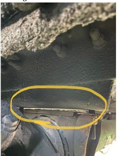
2/10 Ryegate SB detail. An Inspector conducting a Level 1 inspection placed the CMV out of service for a loose pitman arm on the steering gear box output shaft. To view a video of the violation: <a href="https://www.youtube.com/shorts/s-X8YqL8Vlo">https://www.youtube.com/shorts/s-X8YqL8Vlo</a>
