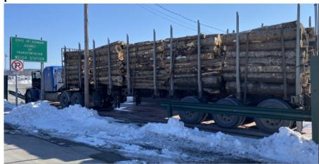
• 2/10 Inspector conducted an inspection on this oversize load at the Colchester detail. The inspection found that the load was 85' 1" long, and the permit was valid for 79' 11". This additional length required a pilot vehicle. Additionally, the boom extended greater than 4' past the rear bumper and was not flagged. The load was grounded until a pilot vehicle arrived and the correct permit was obtained. The carrier was ticketed.
