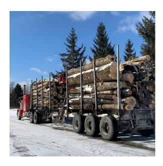
• 3/3 Concord, US Rte 2. An Inspector conducting a Level 2 inspection on a CMV placed the trailer out of service for improper load securement- damaged required web strap. The damage exceeded the limits for a 4-inch strap.
