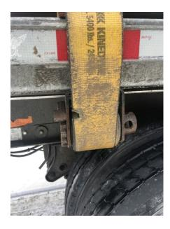
• 3/10 Inspector discovered several sections of damaged synthetic webbing on an oversized load at the Bridgewater detail. The trailer was placed out of service until the straps could be replaced.
