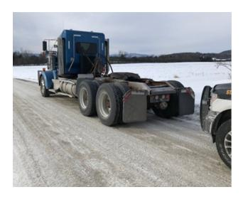
• 1/24 Inspector stopped a dump truck hauling a piece of heavy machinery for a load securement infraction on VT Rte. 2A in Williston. All 4 corners of the machine were not secured as required. The trailer was placed out of service and the driver remedied the defect by attaching additional chains and binders.
