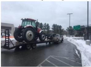
• 12/29 West Danville detail. An Inspector conducting a Level 2 inspection on a five axle CMV placed the CMV out of service for improper load securement.
