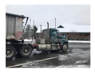
• 12/28 Derby Line Port of Entry detail. An Inspector conducted an inspection on a four axle CMV transporting a piece of machinery. The CMV was operating over its registered weight and required a CDL in that configuration with that weight. The driver was placed out of service for not possessing a CDL Class A and the driver was provided guidance on increasing registered weight.
