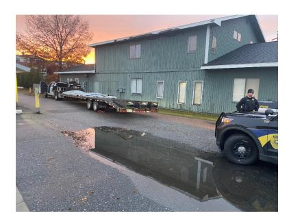
11/12 Inspector inspected a tractor trailer on Rte. 22a in Shoreham. The trailer was placed out of service for no operable brake lamps.
