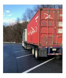
• 12/1 Inspector discovered a vehicle hauling Haz Mat with a steering component that had 1/4" of play at the Ira detail. The vehicle was placed out of service.
