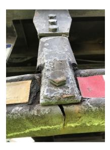
• 11/23 Inspector discovered a crack on the mounting bracket of the sliding trailer plate during a level 1 inspection in WRJ. The defect was documented as a violation only.
